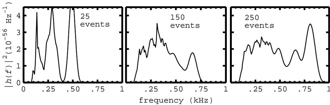
Figure 3: The initial rapid evolution of the GW power spectrum for the first 250 events, equivalent to a time series duration of about 10 s. The first panel shows a bandwidth of about 450 Hz for the first 25 events, equivalent to the first second of the time series. The second and third panels show that significant increases in bandwidth towards higher frequencies occur over the first few hundred events, a result of events occurring at lower redshift.
