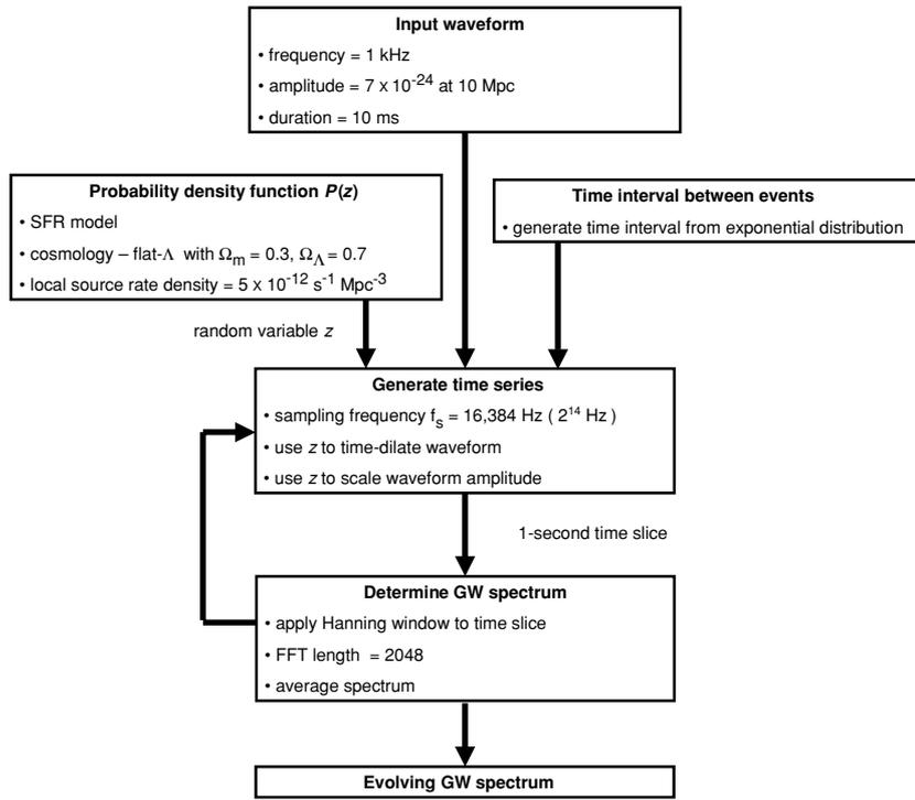
**Figure 6.** Flow chart outlining the simulation procedure for calculating the GW spectral evolution. To produce a time series, the standard input waveform is scaled in amplitude and time dilated according to the random variable  $z$ , obtained from the probability distribution shown in figure 4. As the events are independent, they form a Poisson-distributed time series, with the temporal separations between successive events following an exponential distribution.
